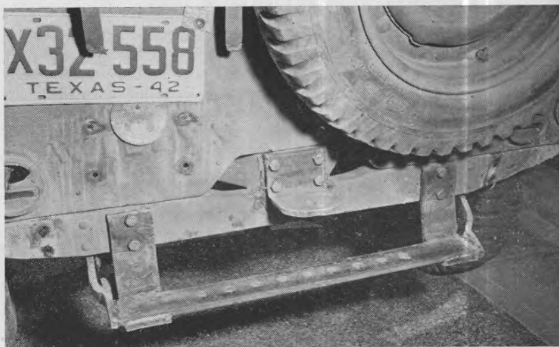
Fig. 2. Drawbar and trailer hitches mounted on military jeep. Either a ball or pin can be used with the trailer hitch.
