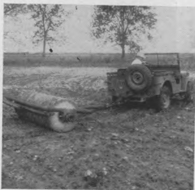
Fig. 8. The military jeep pulling a solid concrete roller weighing approximately 6,000 pounds over fairly firm soil. The drawbar pull was 750 pounds. On soft freshly disked land the pull will be much more.
